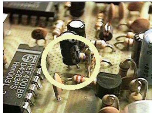
The distance between **TR2 / TR3** body and the PCB must be at least **4mm minimum** and **no greater than 6mm**. 4mm is required for clearance between TR3 and L3.
