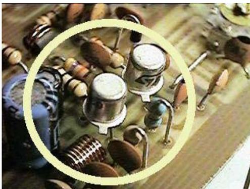
Failure to observe this may cause the collector of TR3 to touch L3 causing a collector-emitter **short circuit**. A good tip is to fit TR2 and TR3 after L3 has been fitted. L3 should be fitted touching the PCB.
