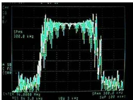
The application of frequency modulation to an oscillator causes a wide range of side-bands to be generated. Each side-band is composed of many carriers, each displaced from the carrier frequency by a multiple of the modulating frequency.
